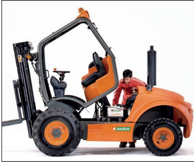
Tilting cab for an easy periodic inspection
